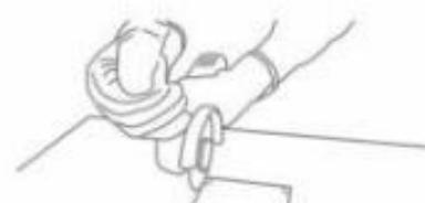
To get internal and L-shaped corners & to reduce the risk of breakage, round off the vertex of the internal corner using bits with a radius of at least 5mm. Then cut with diamond discs, be cautious to stop moving the cutting tool forward. To drill and cut using diamond discs, follow the instructions provided above.
