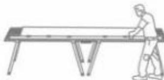
Our products can be cut using diamond discs fitted onto the hand-held electrical grinding machine. The speed of Disc rotation must be high (>10000 RPM) and should have a low feed rate (< 1 m/min). It may be required to cool the disc with water. Recommended discs are the thin types generally used for cutting porcelain stoneware. The surface should be kept on a FLAT base while cutting without any gap underneath.
